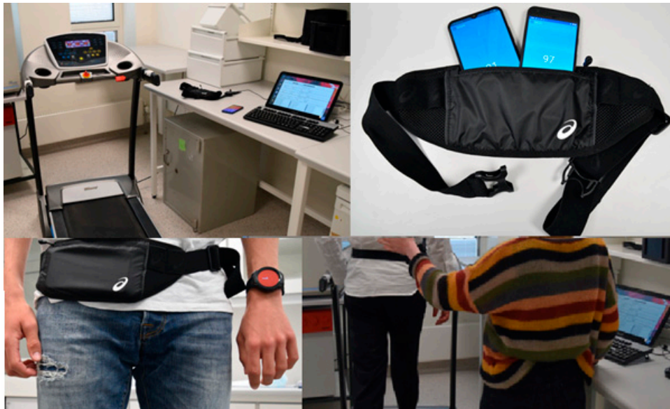
Supplementary Figure S1: Top left, the treadmill which allows for data collection at fixed walking speeds. Top middle, the data collection software, which automatically receives the step count from both phones and allows the observer to manually register observed steps. When reaching 100 steps at a certain speed, the data registration stops automatically, and calculates the differences needed for statistical analysis. Top right the pocket pouch with the two used smartphone models running BeSafe. Bottom left, the pouch affixed to the stomach of the test participants ensuring a standardized measurement point. Bottom right: the test facilitator ensures that the participant is walking steadily and unsupported, ready to stop the experiment if the speed proves too strainful for the participant. Also, the facilitator decides when a steady speed is established, and only when the facilitator starts registering observed steps, by pressing the keyboard will the observed and two measured steps be recorded in real time.
