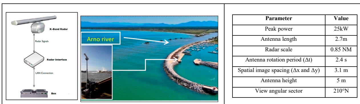
Figure 2. Wave Radar system: hardware architecture on the left. In the middle: photo of the installation site at the port of Marina di Pisa. On the right are the listed Radar system parameters.
