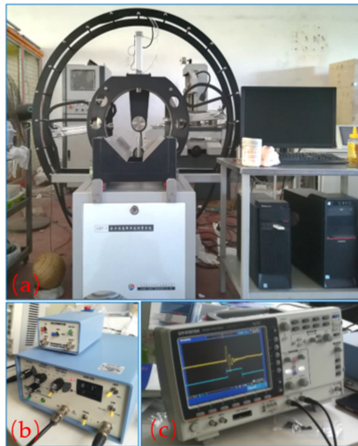
Figure 2. Actual picture of the three-dimensional anisotropic measurement device: (a) omnidirectional positioning system, (b) signal generator and amplifier, and (c) oscillograph.
