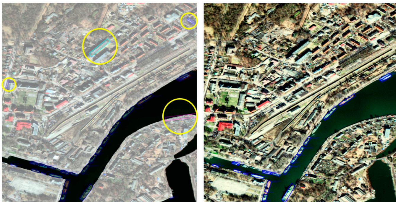
Figure 6. Result of applying FDSESI post-processing. The yellow circle implies false detection on land. The left image implies that the prediction ship of MSD overlaps the area of the sea and land segment mask. The right image implies post-FDSESI.
