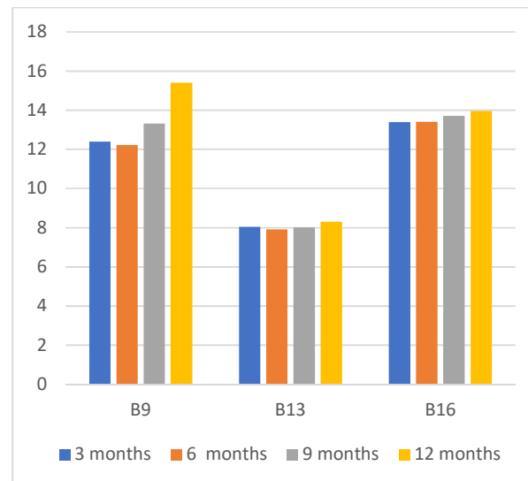
Figure 12. The cross-validated CV(RMSE) values of buildings containing LED retrofit and BMS upgrade ECM.
