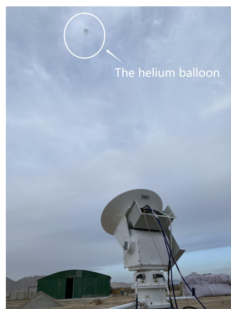
Figure 8. The steerable Cassegrain antenna tracks the air balloon in the ascent stage.
