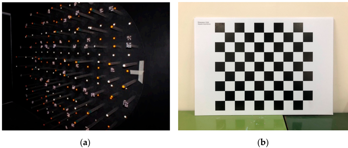
Figure 7. Camera calibration method tools: (a) rotated table with coded targets for the PH method; (b) checkerboard for the CV method.
