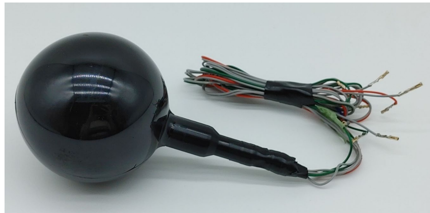
Figure 5. The molded three-dimensional hydrophone.
