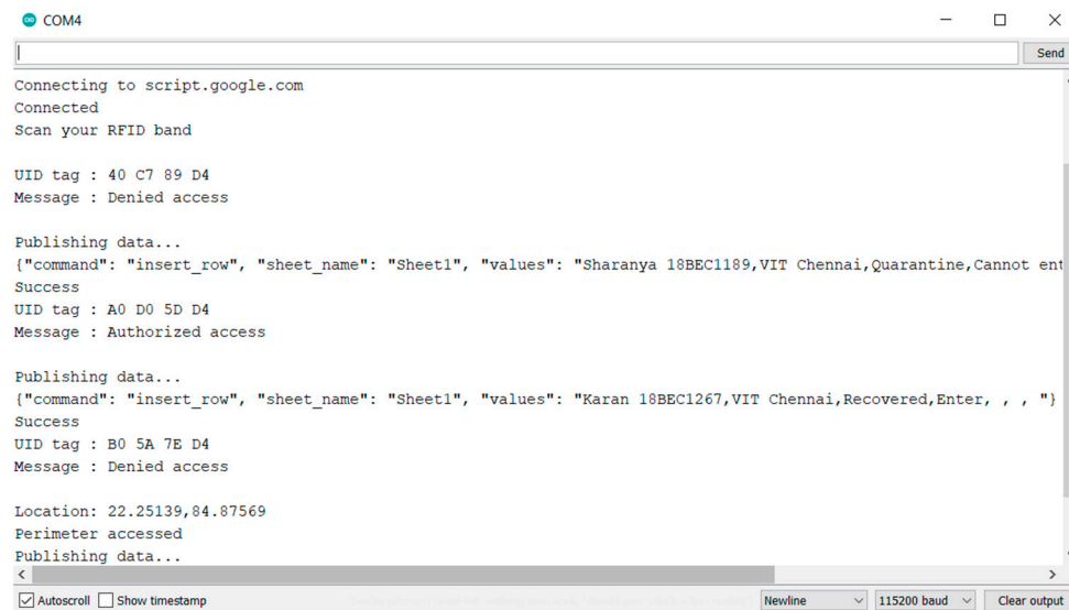
Figure A3. The COM window of Arduino IDE showing the scanning and publishing of user information.
