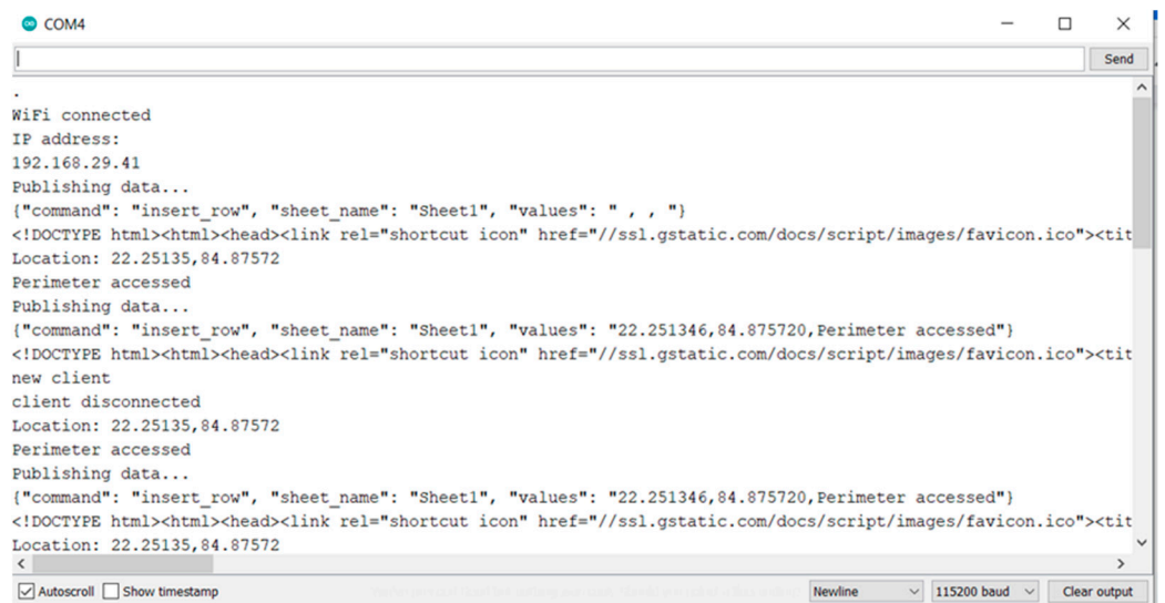
Figure A5. COM window of Arduino IDE showing the publishing of individual GPS data.
