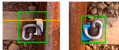
**Figure 4.** Two samples of light loose (X) track fasteners.
