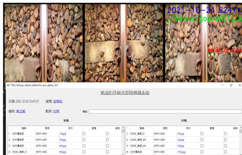
Figure 3. The interface of the track fault detection system.
