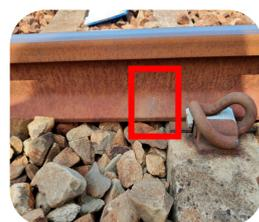
**Figure 15.** Simulated rail break on bottom in side-view.
