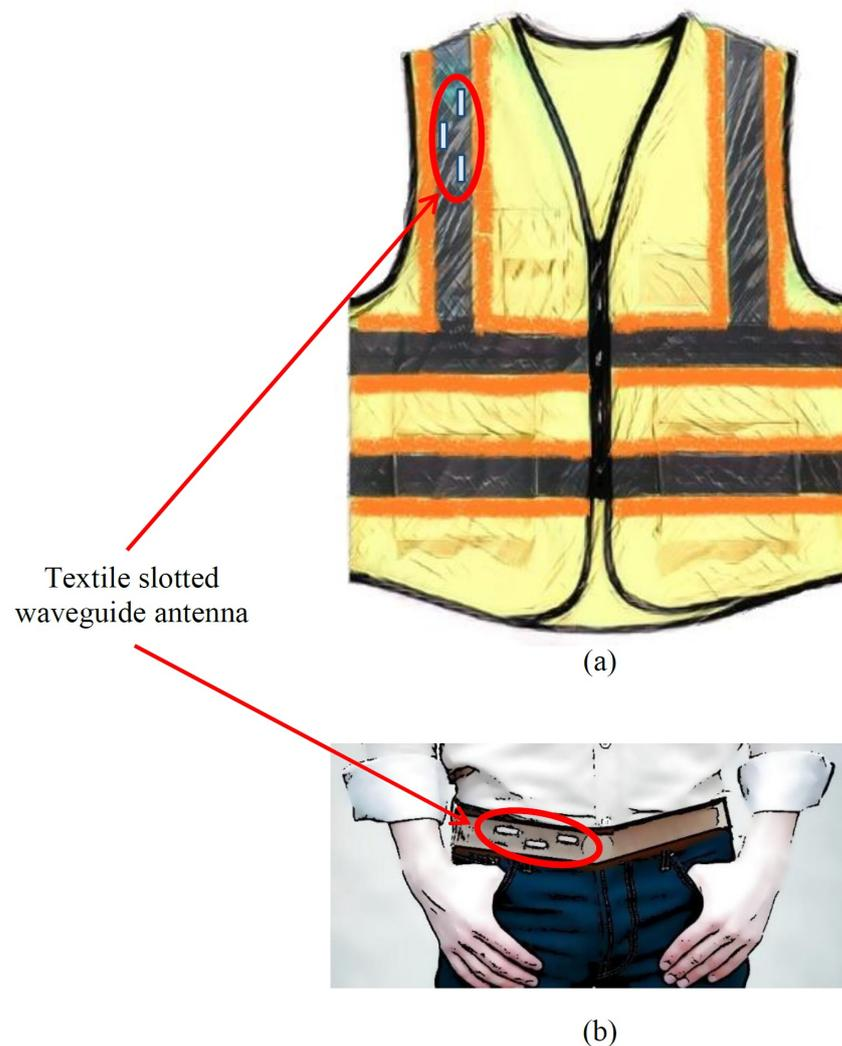
**Figure 8.** The textile antenna in use: (a) Smart safety vest, (b) smart belt.
