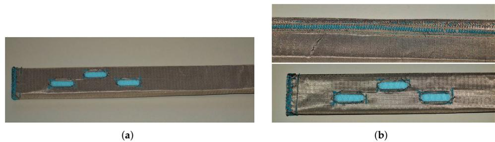
**Figure 3.** Prototype of the textile antenna (a) and details of sewing the waveguide, slots, and short-circuit (b).
