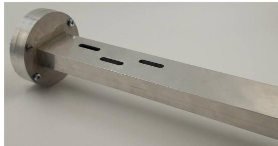
**Figure 4.** Prototype of the aluminum antenna.
