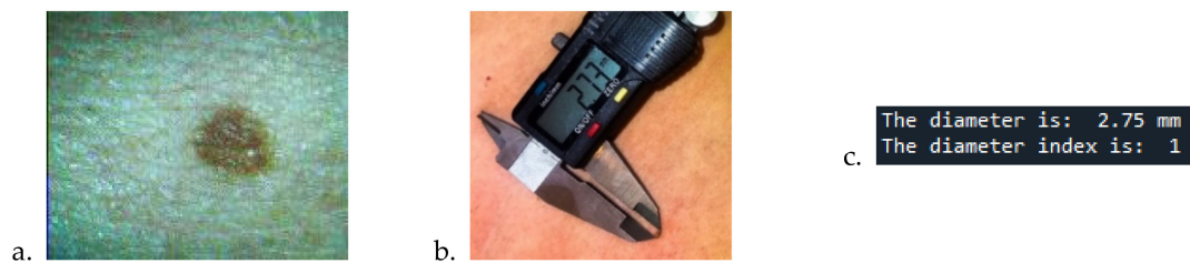
Figure 8. Mole diameter analysis for an image: (a) captured by the camera, (b) measured by vernier, (c) by calculating the diameter index.
