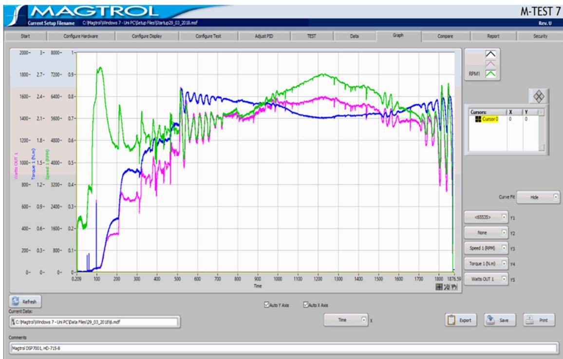
Figure 2. Evolution of the Saito FG-40 engine during an experimental dynamometer run.
