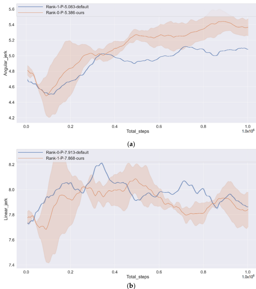
Figure 9. CAV changes in steering angle and linear acceleration during driving. (a) Angular jerk; (b) Linear jerk.
