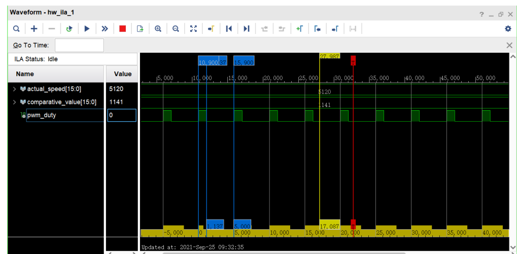
Figure 24. Embedded logic analyzer (ILA) acquisition signal diagram.
