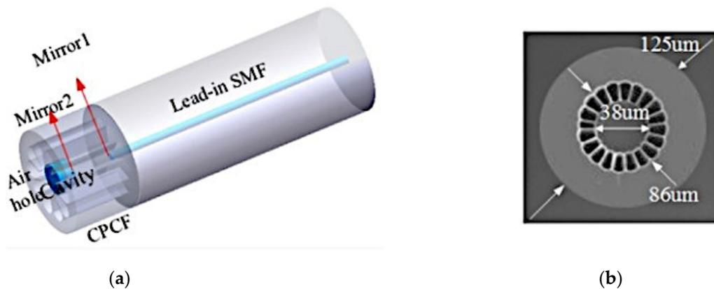
**Figure 7.** (a) Schematic structure of the concave-core PCF FPI sensor. (b) Microscopic cross-sectional view of the CPCF. Reprinted/adapted with permission from [36]; © The Optical Society.
