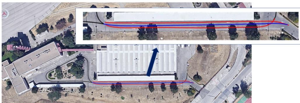
Figure 7. Vehicle trajectories in the parking lot (blue: S1; red: S2; black: common).
