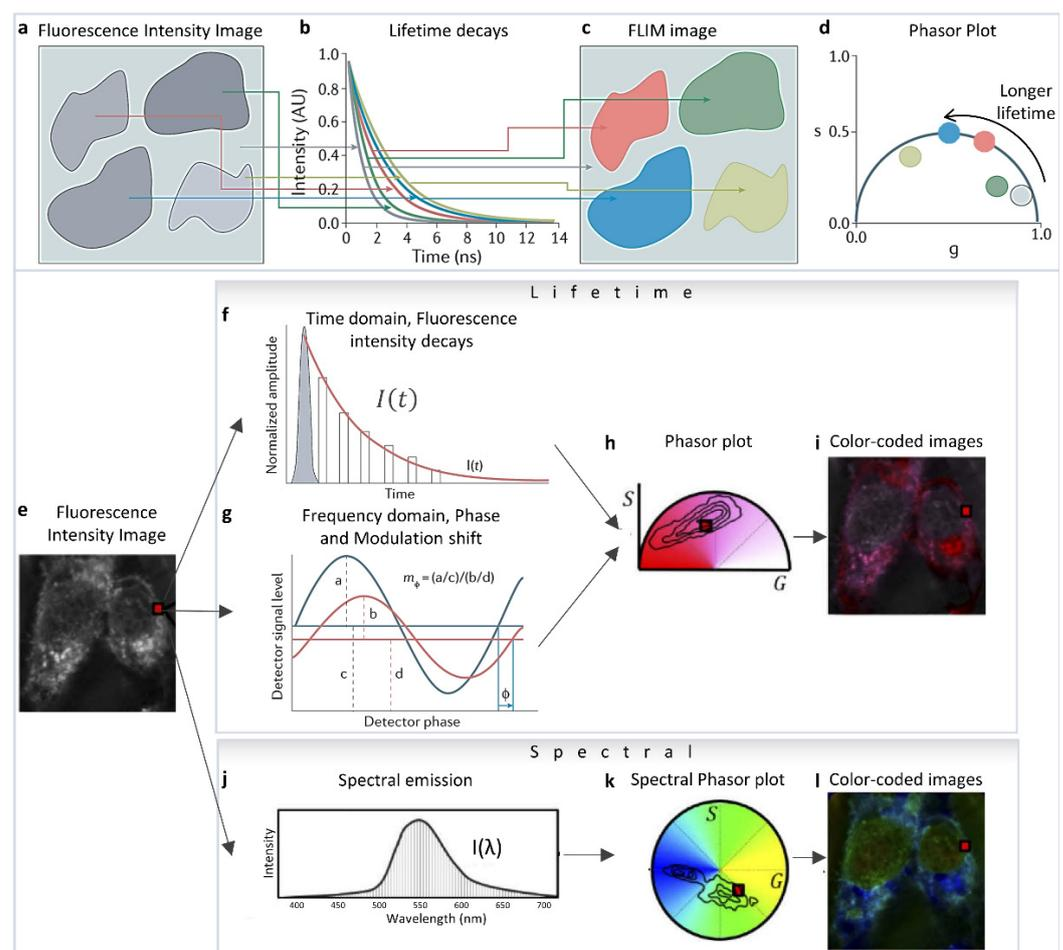
**Figure 1.** Phasor transformation. (a) Fluorescence lifetime imaging microscopy (FLIM) measures the fluorescence lifetime decays in different parts of the image (b), and color-codes areas (c) according to their decay times (b) or their phasor clusters (d). The resulting phasor plot (d) represents species
