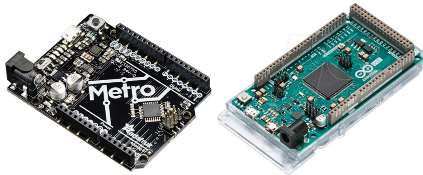
Figure 13. Adafruit Metro (left) and Arduino Due (right) are two of the Arduino boards compatible with the PPG EduKit.
