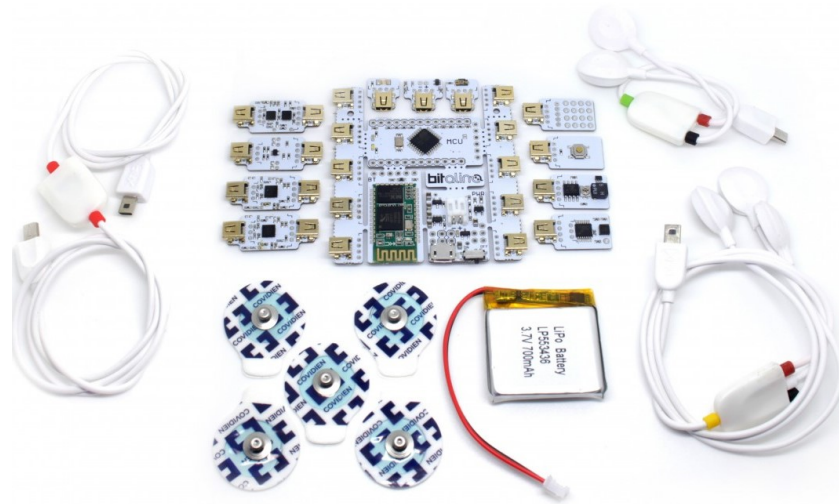
Figure 6. BITalino (r)evolution Plugged Kit BLE/BT. The motherboard with some of the attachable sensors is shown.
