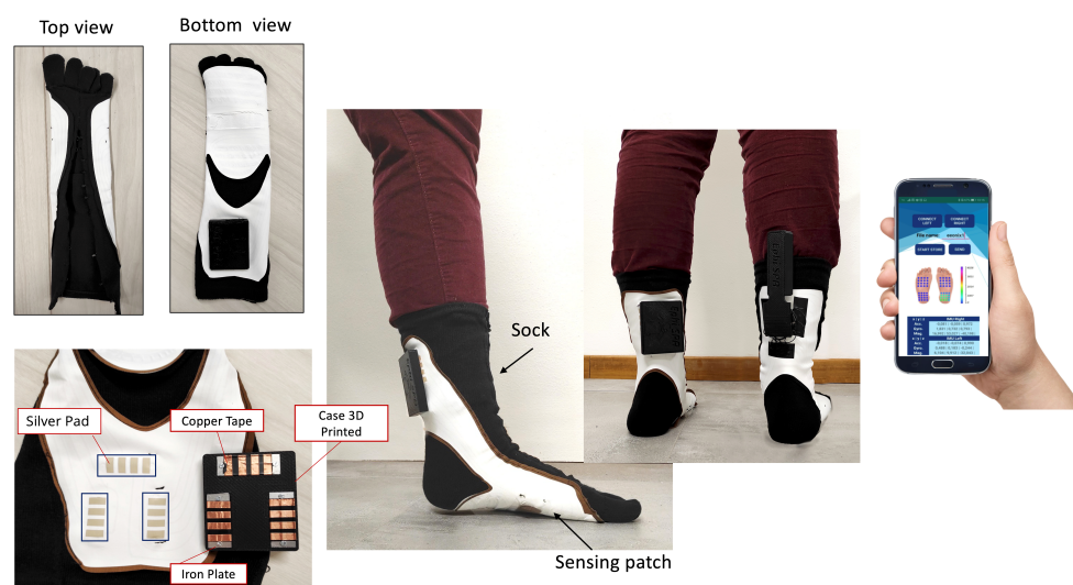
Figure 4. The sensorized sock prototypes. The left side of the figure shows the prototype details, highlighting the location of the 12 electrical connections (3 blocks of 4 silver pads) and the electronic unit with the dedicated magnetic connector. The picture on the right shows the main screen of the developed mobile application.
