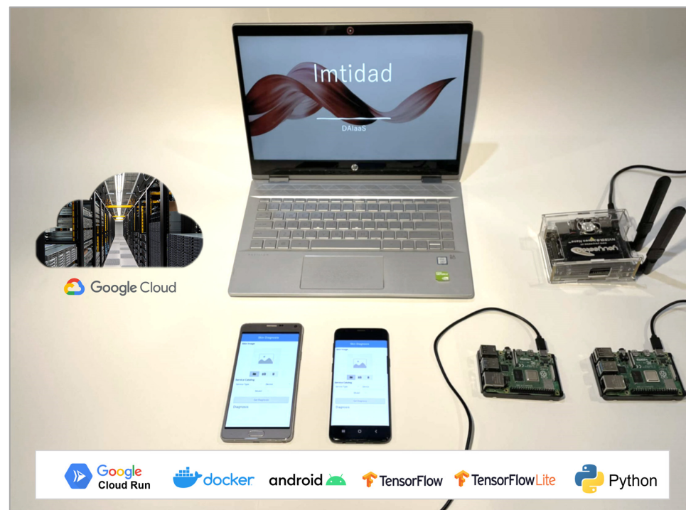
Figure 7. Imtidad testbed: devices and platforms.
