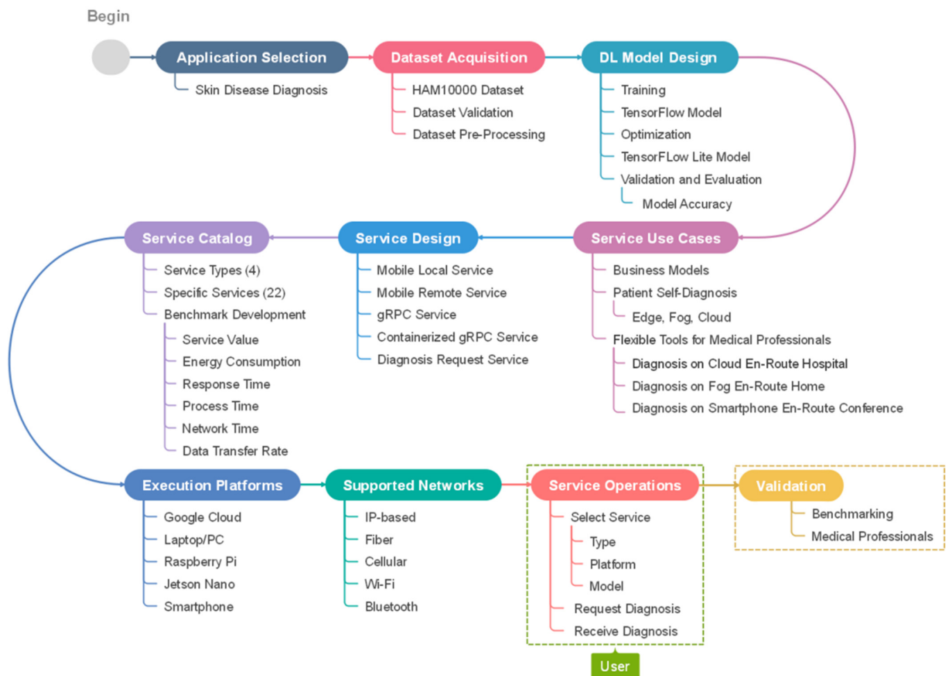
Figure 3. Workflow Diagram for creating a skin disease diagnosis catalog refined from Imtidar Reference Architecture.
