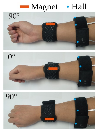
Figure 8. The relative position between magnet and hall at different wrist angles.
