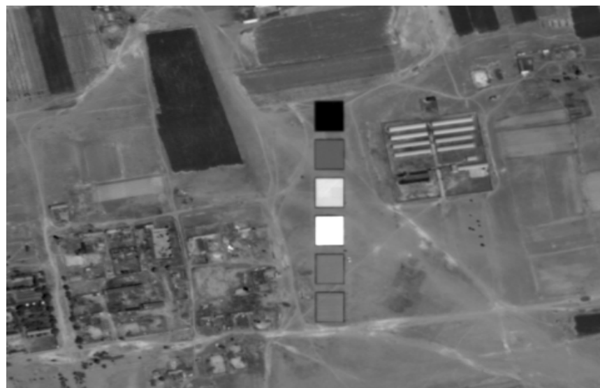
Figure 4. The arrangement of the calibration tarps at the RadCalNet Baotou site.
