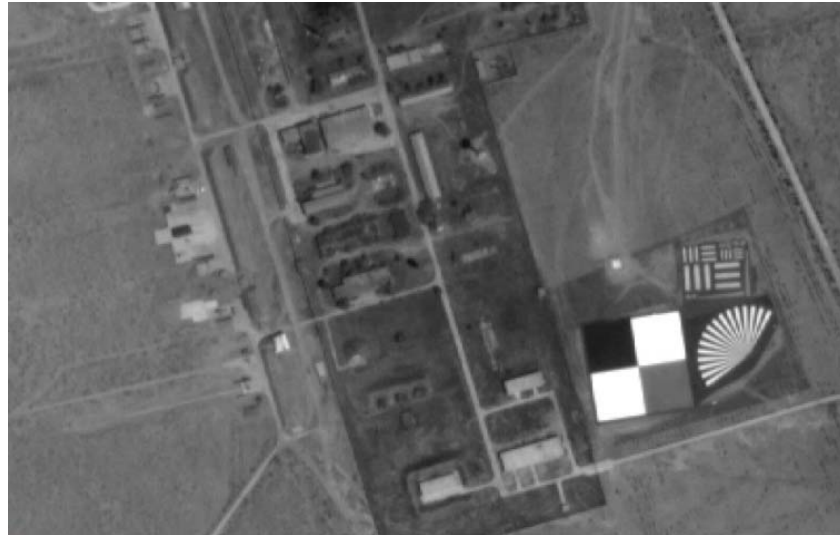
Figure 3. The gray-scale permanent artificial targets at RadCalNet Baotou site.
