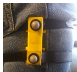
Figure 1. Attachment of IMU to the reference thigh of the subjects.
