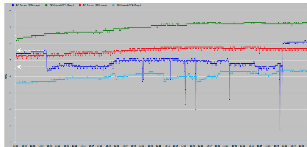
Figure 17. Effect of induced shading on SP1 from 12:30 to 13:55.
