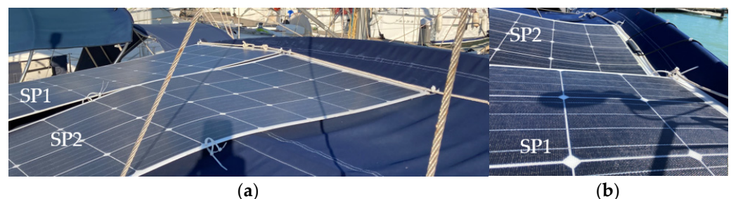
Figure 13. Projection of (a) backstay and (b) antenna shading lines on SP1 and SP2 in the early hours of the day (9:30 a.m.).
