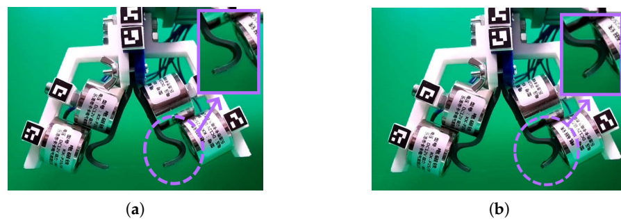
Figure 10. The soft gripper reaction on electromagnet. The upper pair of electromagnets turned on (a). The both pairs of electromagnets turned on (b).
