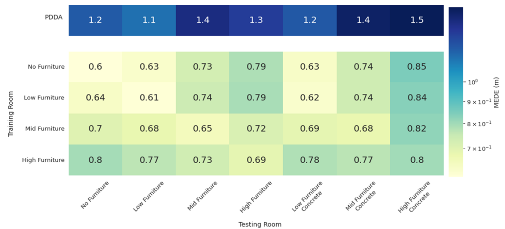
Figure 7. MEDE of the CNN-based joint model on different rooms. PDDA methods performance in each room is included for reference.
