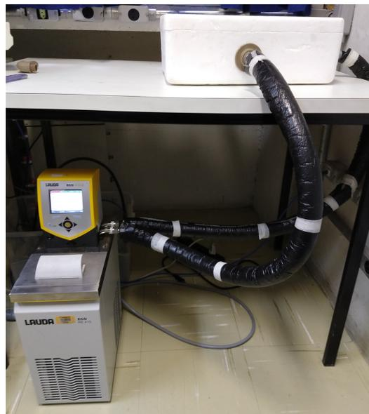
**Figure 1.** Experimental apparatus used in the tests to determine the temperature dependence of the sound speed. The setup consists of a thermostatic bath, capable of promoting the external flow of temperature-controlled fluid, and a container where the thermal exchange happens.
