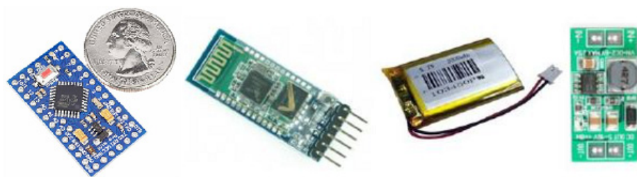
Figure 7. Arduino Mini, HC-05 Bluetooth module, iOptron Lithium-Poly 3.7 V battery, and the step-up DC-DC converter.
