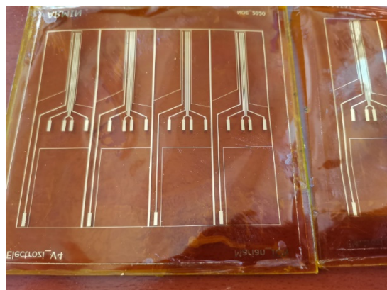
Figure 9. Electrodes used as samples for the bending tests.
