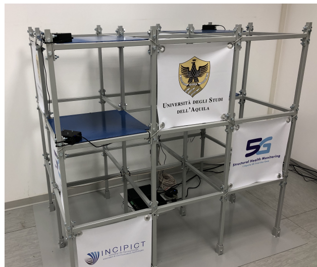
Figure 5. Test frame equipped with sensor boards and connected to a 5G CPE.
