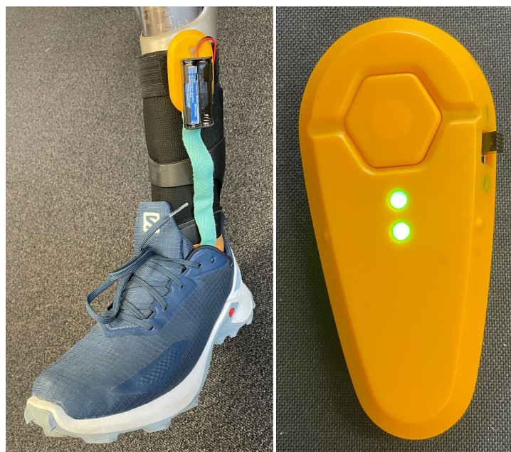
Figure 1. The Suralis sensor systems: The sensor sock worn on a prosthesis within a shoe including the transmitter unit (left). The IMU integrated in a housing together with the transmitter unit (right).
