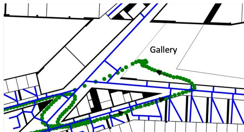
Figure 10. Part of the trajectory of the *eight* path, that wrongly proceeds in the “gallery”, when using the weighting by routing support method, where black arrows indicate the walking direction and the green points represent the position estimates for each step.
