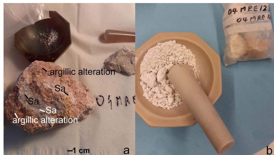
Figure 2. (a) Rock specimen 04MRE123, selected for clay extraction, where the occurrence of sanidine and argillic alteration is shown. (b) Hammered rock pieces in the agate mortar before X-ray diffraction, whole-rock measurement and clay extraction procedure.
