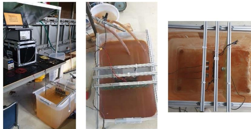
Figure 5. Accelerated corrosion experiments setup.
