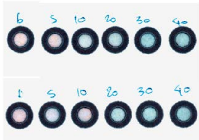
Figure 4. Color alteration for calcium determination according to the method, in the concentration range between 5 and 40 mg L -1 , visible even to the naked eye.
