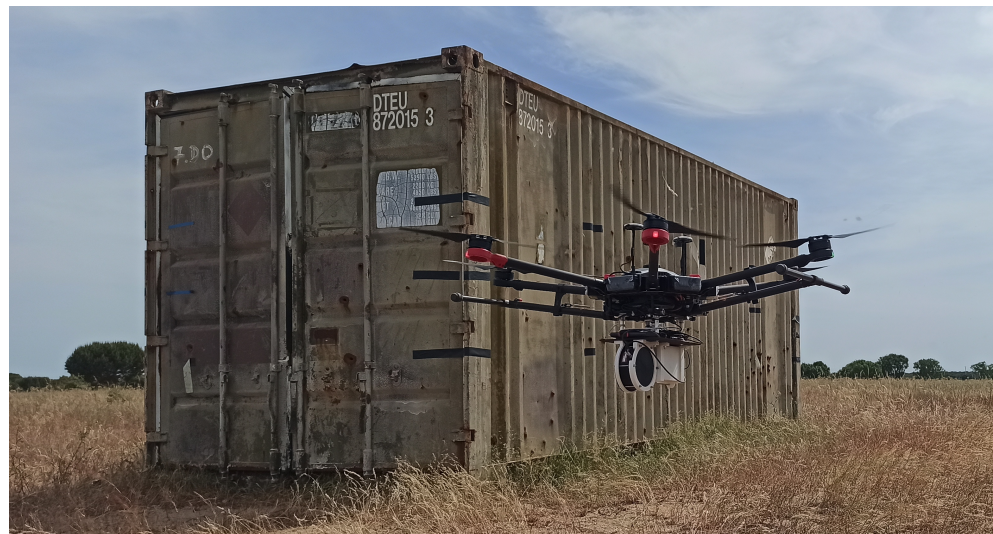
Figure 11. Multirotor with developed radiation detection system screening a shipping container cargo.
