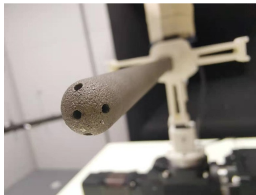
Figure 4. Five-hole probe made by 3D metal printing.
