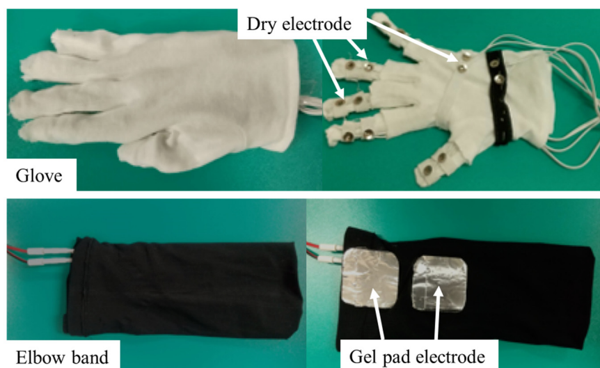
Figure 8. The electrode layout inside the haptic glove.
