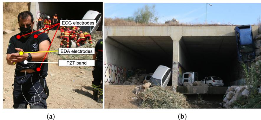
**Figure 8.** Real-time monitoring exercise: (a) deployment of bio-signal measurement devices on first responder in the initial area of operations; (b) tunnel entrance. Left side entrance was used.
