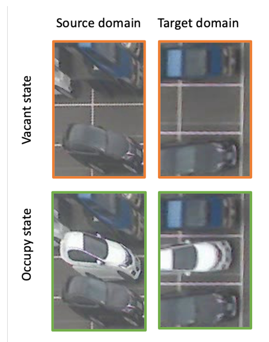
Figure 2. Vacant and occupied samples [12] on source and target domains. They are collected at the same slot and belong to a trajectory [18]. Each row represents samples at the same slot but from different domains. Each column represents samples in a trajectory where the background is similar, but the differences are from the object at the middle slot.
