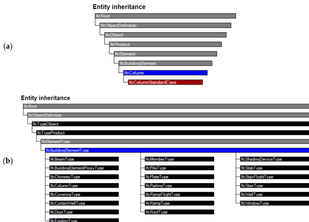
Figure 10. IFC entities classification and their inheritances: (a) The entities inheritance focused on specific standard elements; (b) The inheritance focused on different building element types (BuildingSMART).
