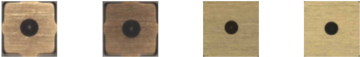
Figure 6. Samples images of non-defective or good epoxy drop substrate.
