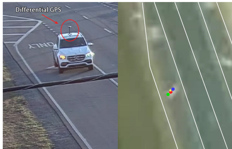
Figure 6. Vehicle equipped with a differential GPS receiver and its location in an aerial view map.
