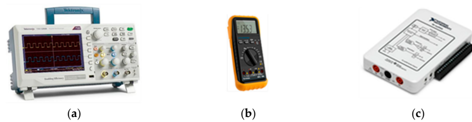
Figure 5. Measurement equipment: (a) oscilloscope; (b) multimeter; and (c) NI myDAQ.
