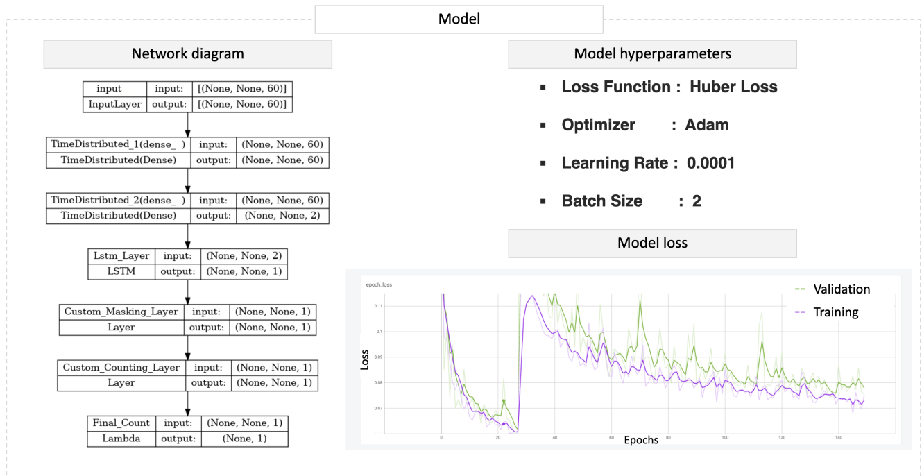
Figure 4. From left to right, this image presents the network’s diagram of the counting model with the input (60 acceleration signals) of variable length and output of 1 number. Moreover, the hyperparameters include Huber loss, ADAM optimizer, a learning rate of 0.0001, and a batch size of 2. An example of a learning curve for the training and validation sets demonstrates the model’s performance during training. The x -axis represents the number of training epochs, while the y -axis represents the loss metric.
