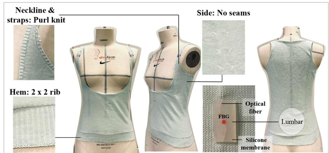
**Figure 6.** Seamless knitted undergarment created using Shima Seki knitting machine, and silicone-embedded FBG sensor inlaid in the warp direction.
