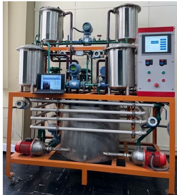
Figure 1. Quadruple tank system of the PUCP's Advanced Control Systems Laboratory.
