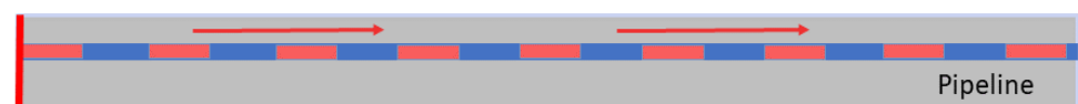
Figure 14. The sensor system is configured as a fiber sensor that covers the pipe, with the measurement units evenly distributed along its length.
