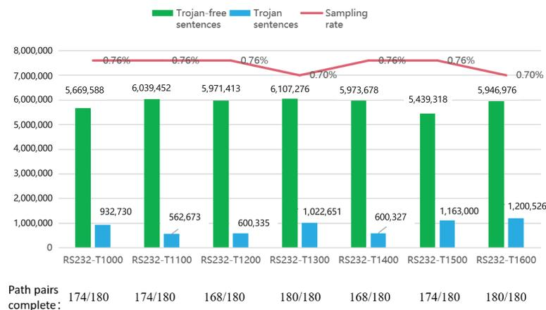
**Figure 6.** Complete extraction rate, label statistics, and sampling coverage in seven netlists.
