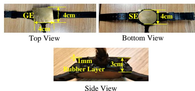
**Figure 6.** Electrodes used in the physics experiments.
